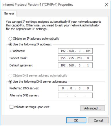
This image is for a PC running Windows 10. To get to the TCP/IP properties screen, go to: Control Panel->Network and Sharing Center->Local Area Connection->Properties. Select Internet Protocol Version 4(TCP/IPv4) from the scroll box and click Properties. That gets you to the dialog box shown left.
